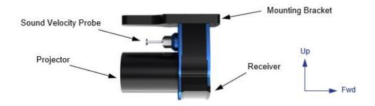
The sensors must be mounted rigidly and free from vibration, and there must be no independent movement between sensors. For Baywei M5, the GNSS antennas must have a clear sky view. It is recommended to separate the GNSS antennas by a distance of 2m.
